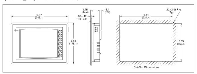
Figure 10. HMI08CE — Approximate Dimensions in Inches (mm)
